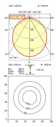
Light sourceLEDWork equipmentWithoutConnected load22 - 26 V; DCPower consumptionca. 16 WLuminous fluxapprox. 1.450 lmLuminous efficiencyapprox. 90 lm/W
