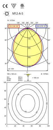
Light source LED Work equipment Without Connected load 22 - 26 V; DC ca. 15 W **Power consumption** Luminous flux approx. 1.575 lm Cold white Light type/-color Colour temperatur approx. 5.000 K Color rendering index CRI ≥ 80 Direct **Light distribution** 89° / 97° Beam angle **Chromaticity tolerance LED** < 4 SDCM Glare control Screen System of protection IP 54
