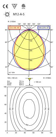
Light source LED Work equipment Without Connected load 22 - 26 V; DC ca. 30 W **Power consumption** Luminous flux approx. 3.150 lm Cold white Light type/-color Colour temperatur approx. 5.000 K Color rendering index CRI ≥ 80 **Light distribution** Direct 89° / 97° Beam angle **Chromaticity tolerance LED** < 4 SDCM Glare control Screen System of protection IP 54
