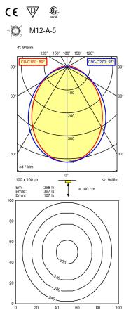
light source LED work equipment without connected load 22-26 V, DC env. 7,5 W power consumption luminous flux approx. 945 lm luminous efficiency approx. 126 lm/W light type/-color cold white colour temperatur approx. 5.000 K CRI > 80 color rendering index light distribution direct beam angle 89° / 97° chromaticity tolerance LED < 4 SDCM glare control screen system of protection IP 54 class of protection
