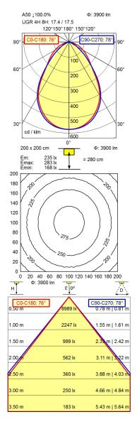
Work equipment Electronic ballast **Connected load** 220 - 240 V; 50 Hz; 60 Hz Power consumption ca. 30 W Standby ca. 0,5 W Power factor env. 0,900 Luminous flux approx. 3.900 lm Luminous efficiency approx. 130 lm/W Light type/-color Warm white Colour temperatur approx. 3.000 K Color rendering index CRI ≥ 80 Light distribution Direct **Direct ratio** approx. 100 % Beam angle 76° / 78°
